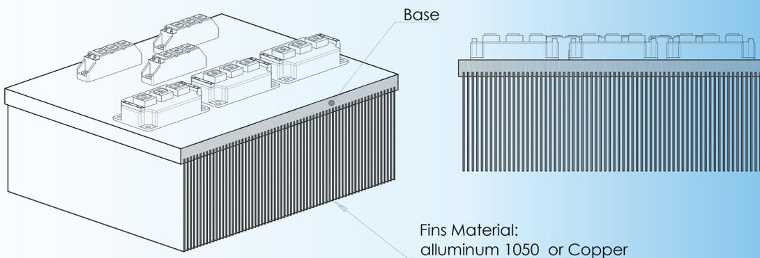
Heatsink base and fins can be made using alluminu 1050 or copper, however is still possible to have a combination of both
