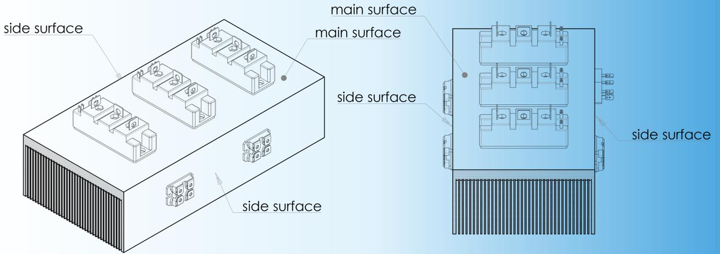
**Example EV-B SERIES heatsink (open profile) with components to be dissipated assembled on 4 sides**
