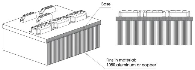
The fins and the base can be in 1050 aluminum or copper it is also possible to have a combination of the 2.
